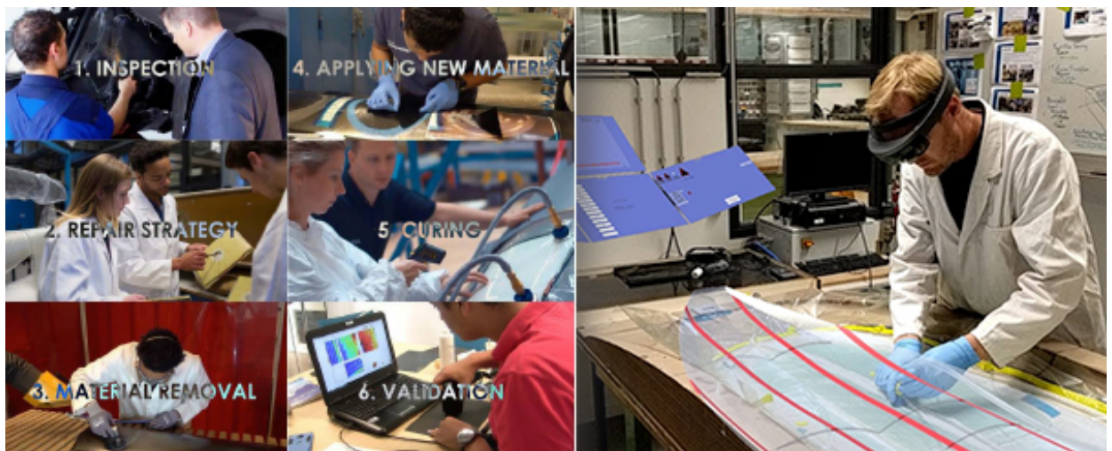
Figure. 2. FIXAR, applying new ways of automation for repairing composites for the windenergy and aviation industry (ref: Inholland Composites).
