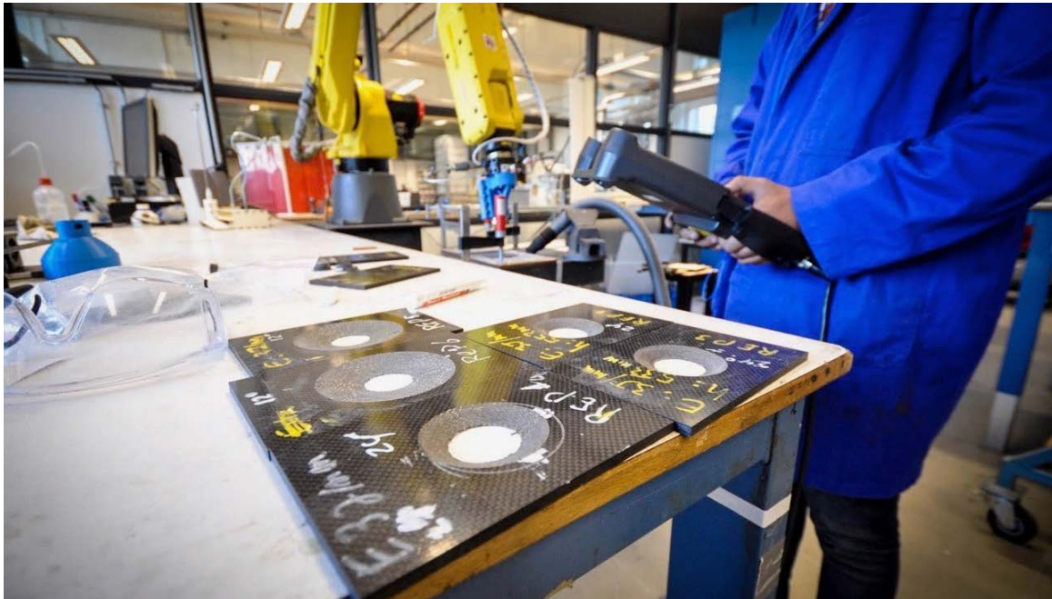
Figure 3 Experimental setup at Inholland Composites for Robotic Scarf Repair on carbon laminates
